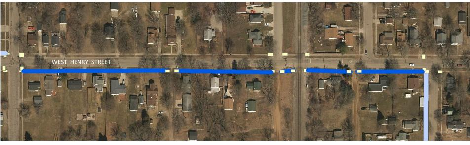
NOTE: SIDEWALK TO END 8 FT. FROM END OF RAILROAD TIES. NO FURTHER THAN 16 FT. FROM THE END OF THE RAILROAD TIES, PLACE 24" WIDE ADA TRUNCATED DOMES ACROSS THE FULL WIDTH OF THE SIDEWALKS.
